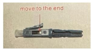
**Step 6**: Insert the glass into the fiber optic connector. Make sure the optic fiber is slightly curved.
